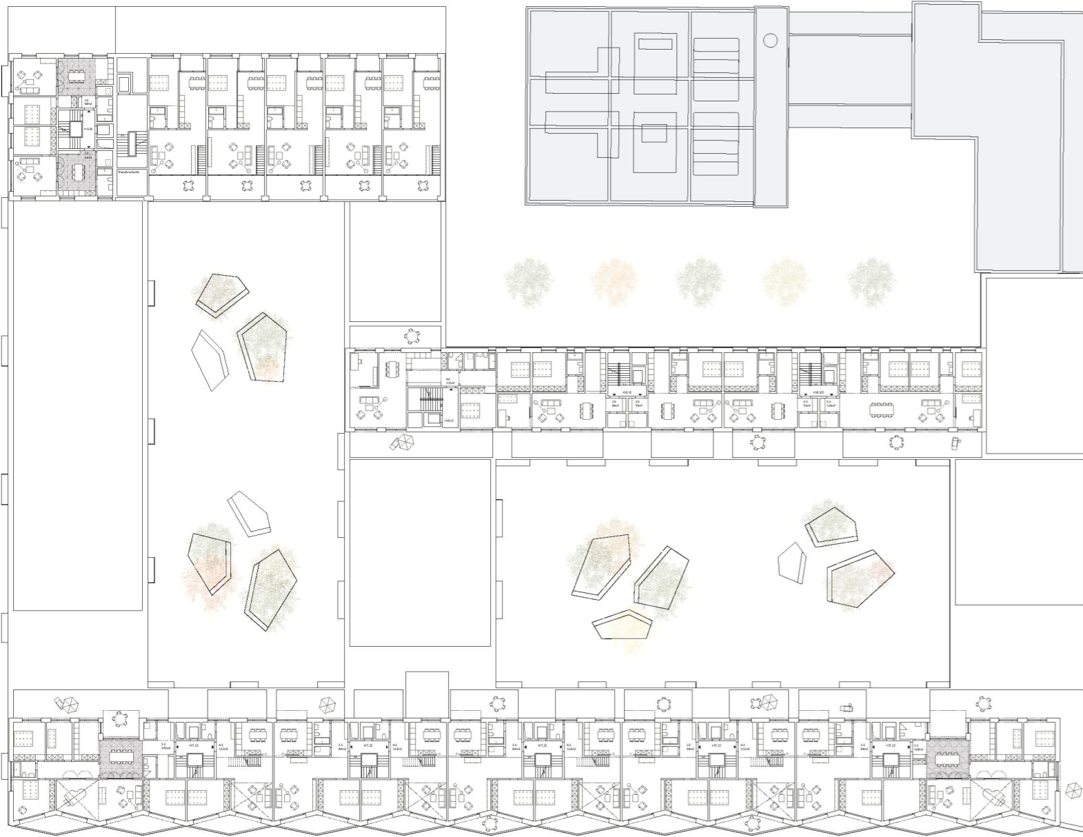
Perimeter Ost - Grundriss 5./6. Obergeschoss (OK = +17.23 / +18.13) 1:200
